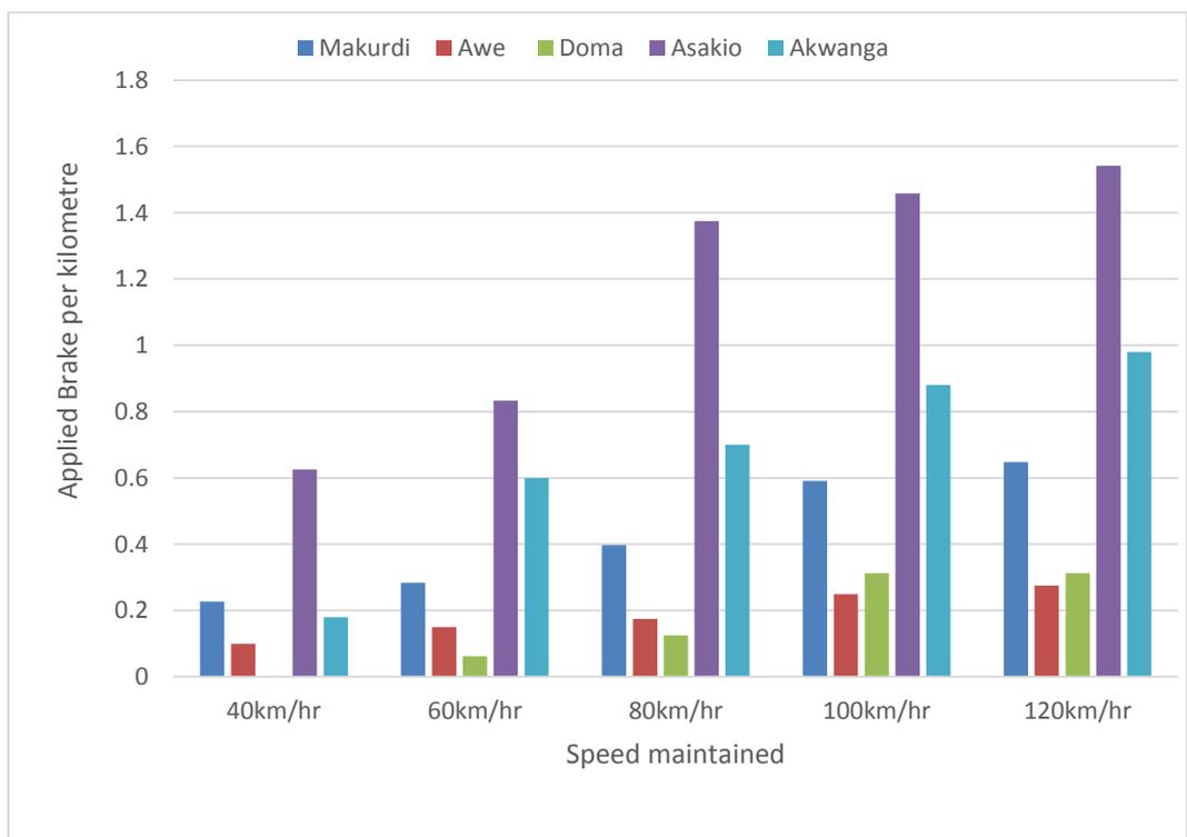
**Figure 1** Pictorial display of average number of brakes applied per kilometre *versus* speed. The correlation between these two variables is positive for the entire speed range.
