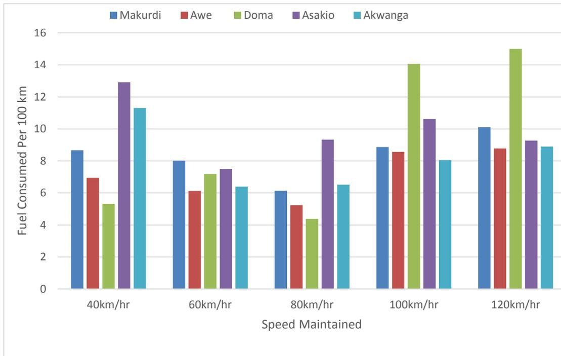
**Figure 2** This clustered column gives the pictorial relationship that was obtained from the experiment; this corresponds with figures obtained from fuel economy database for Toyota Corolla model.
